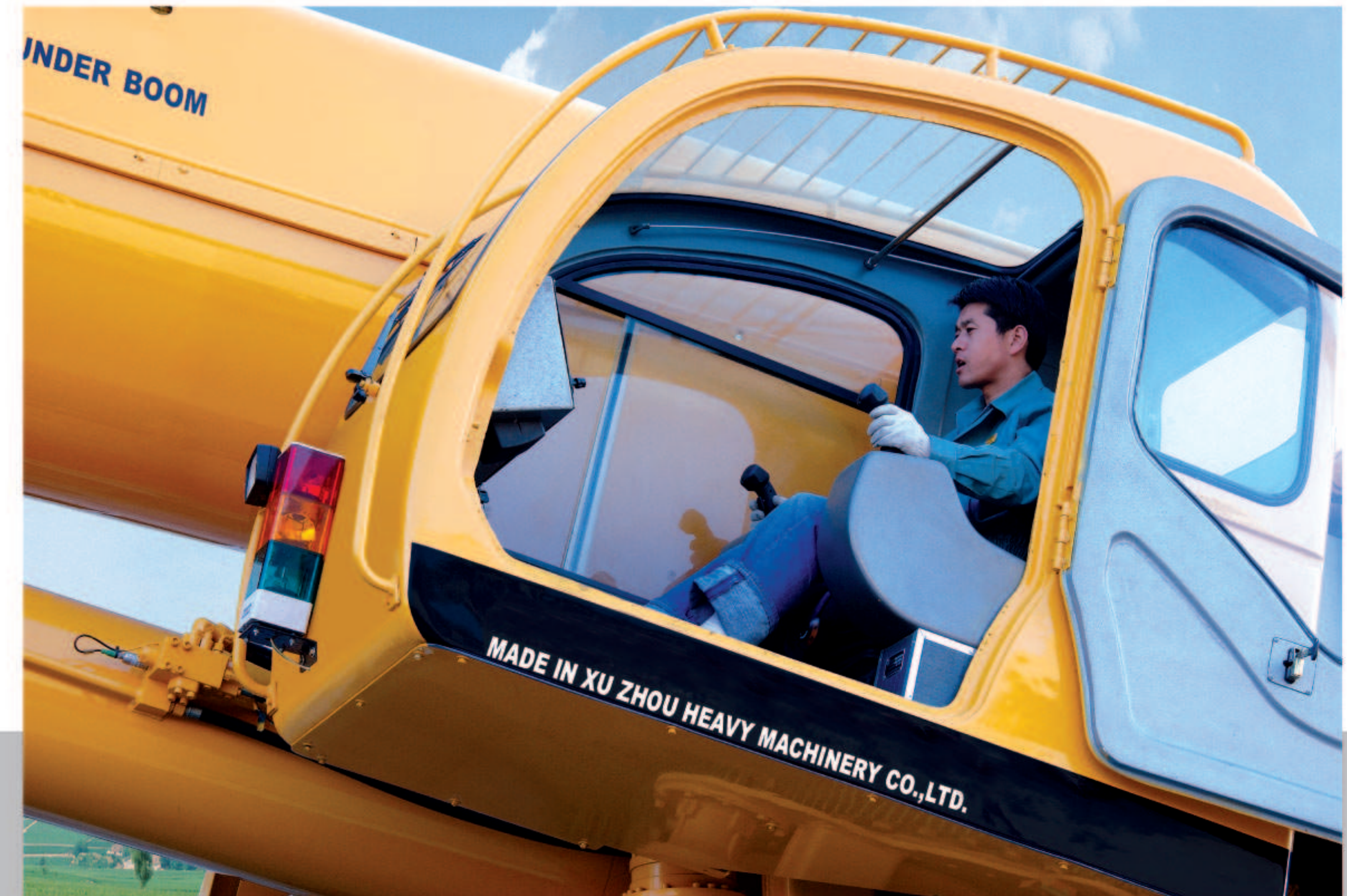
Streamlined upper cabin cab made of compound material can be tilted backwards 20°
